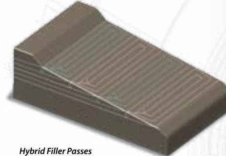
Hybrid Filler Passes combines waterline and scallop toolpath motion.
